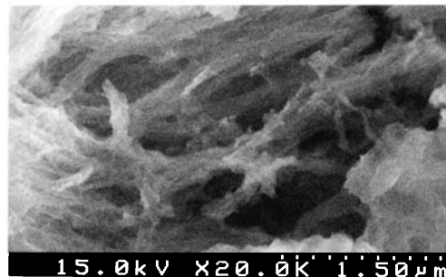
Figure 1. SEM picture of a xerogel obtained from 2a in dichloromethane (0.0162 mol dm -3 ) at -110 °C/0.1 torr.
